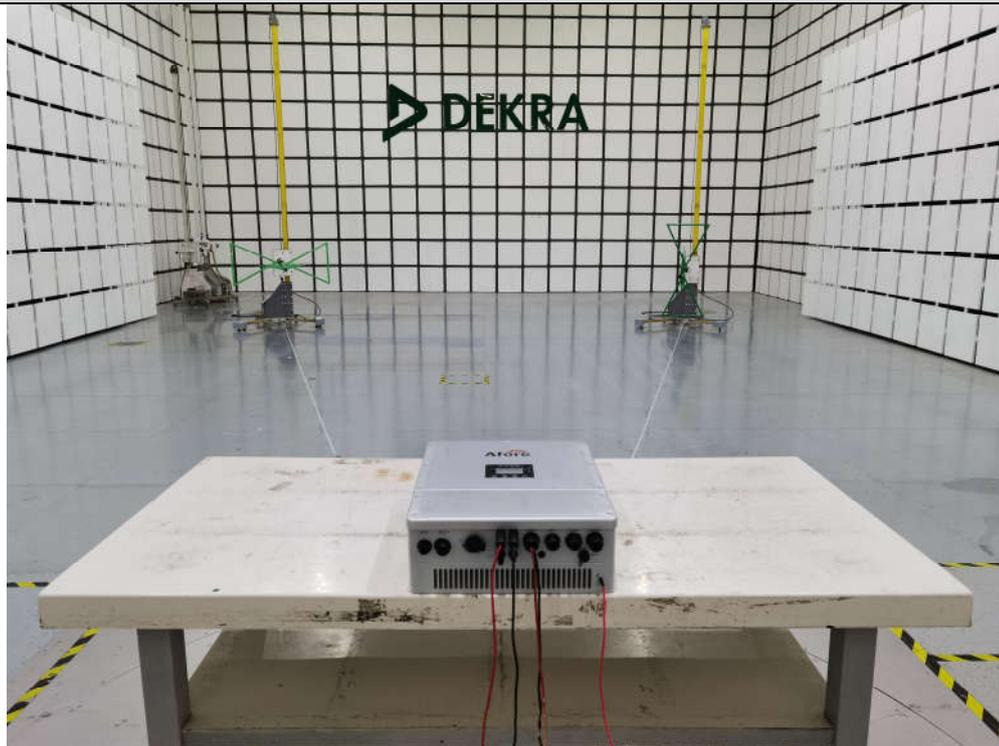
**Radiated electromagnetic disturbances (30 MHz to 1000 MHz):Back View**
