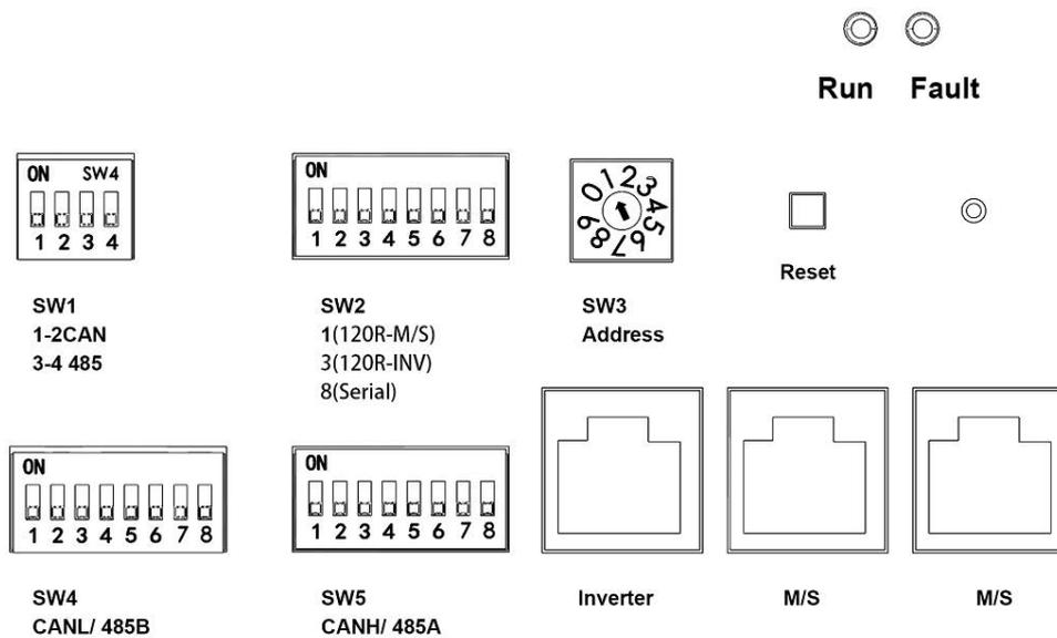
Confirm that the CANL/485B DIP switch is set to SW2 which pin is used for CAN high signal by inverter (4-CANH/485A), and the CANL/485B DIP switch is set to SW1 which pin is used for CAN low signal by inverter (5-CANL/485B).
