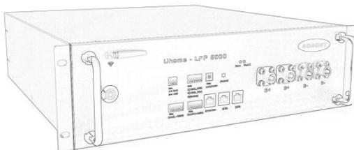
Press and hold the panel button for about 4s and then release it after the two LED lights on, measure the voltage at the terminal interface with a voltmeter. If the voltage is lower than 48 V, do not use the battery and contact AOBOET hot line or your distributor.
