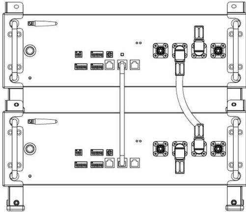
Feed a data cable to M/S communication terminal interface one by one directly.
