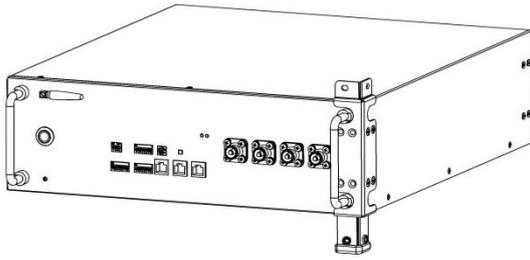
1. Fix the braced feet to battery's mounting holes one by one.
