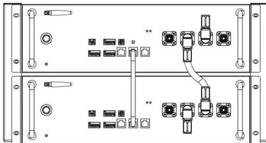
For wall mounting, the battery Series connection number should be less than 4, if more batteries installed, a cabinet was recommended.
