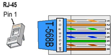
If needed, the network cable should be made like that diagram. But the network cable between battery and Inverter should be made following the definition of Inverter. If available, use a LAN cable tester to check whether the cable is faulty.
