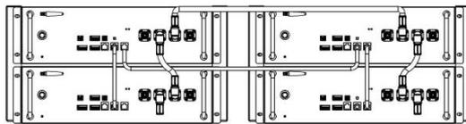
**NOTICE** If battery connected in Series mode, it's better to be installed in Ground installation method, for the Power cable resistance difference between stack and battery pack, which will have fade effect on voltage balance.
