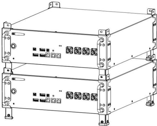
2. If more power and energy needed, two or more (less than 4) batteries could be installed in one stack.
