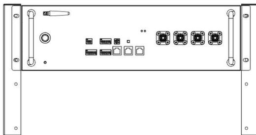
For wall mounting, the battery Series connection number should be less than 4, if more batteries installed, a cabinet was recommended.
