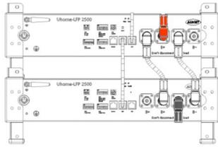
For parallel installation, please pay attention on Cable connection, and the DIP8 of SW2 no need to be changed and stayed on Initial Factory state.
